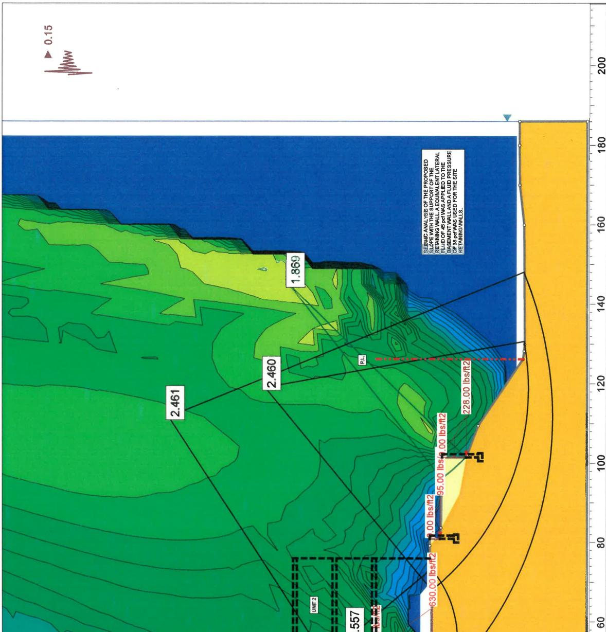
SEISMIC ANALYSIS OF THE PROPOSED SLOPE WITH THE SUPPORT OF THE RETAINING WALL. A EQUIVALENT LATERAL LOAD OF 45 psf WAS APPLIED TO THE SANDFEE BRECCIA. THE SEISMIC COEFFICIENT OF 35 pct WAS USED FOR THE SITE RETAINING WALLS.
