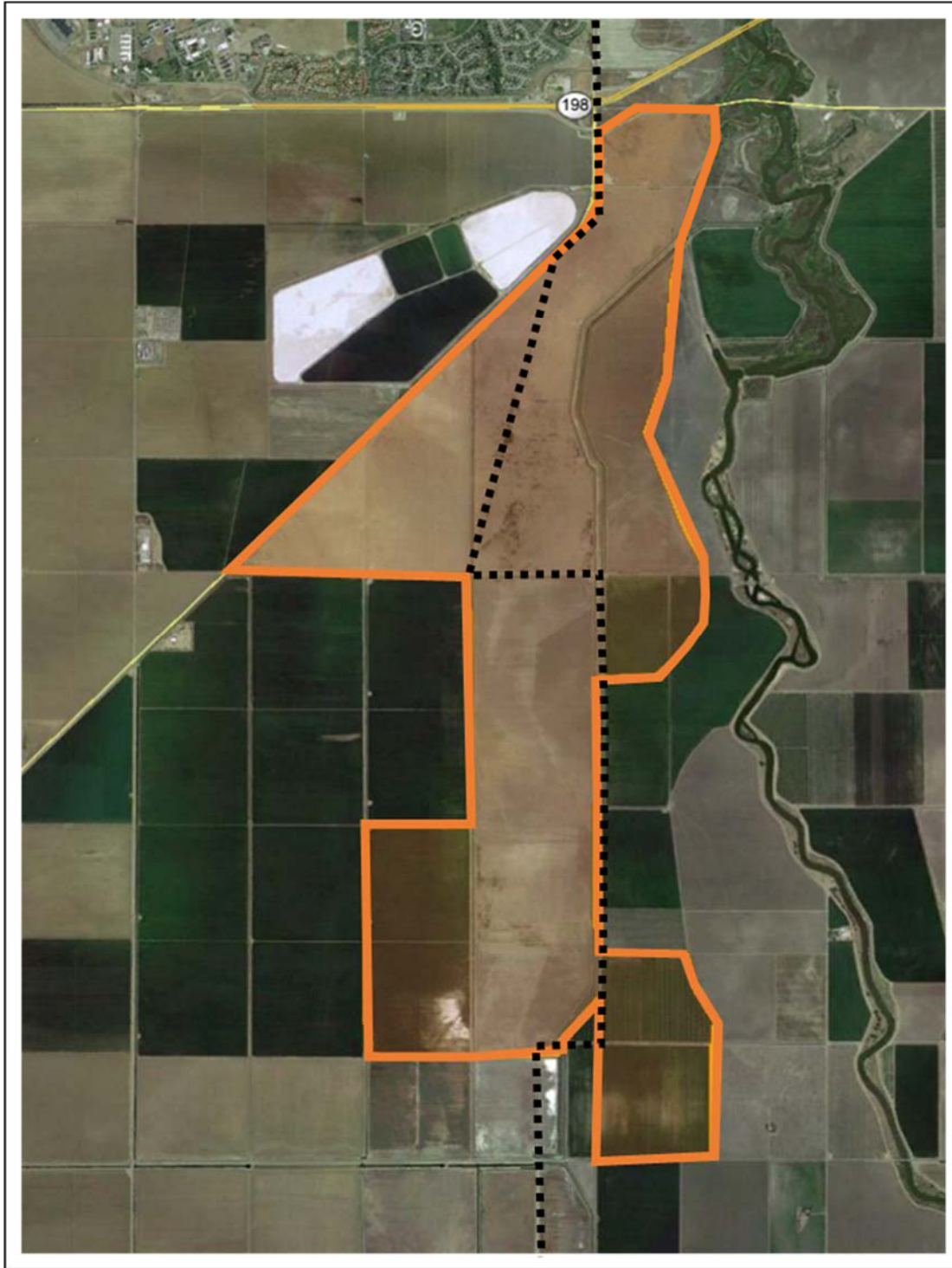
Figure 2-1 Groundwater subbasin boundary near the proposed RE Slate project area. The orange outline shows the RE Slate project site. The dashed black line shows the boundary between the Westside (to the left of the figure) and Tulare Lake (to the right of the figure) groundwater subbasins of the San Joaquin groundwater basin, as defined by CA DWR in 2016.
