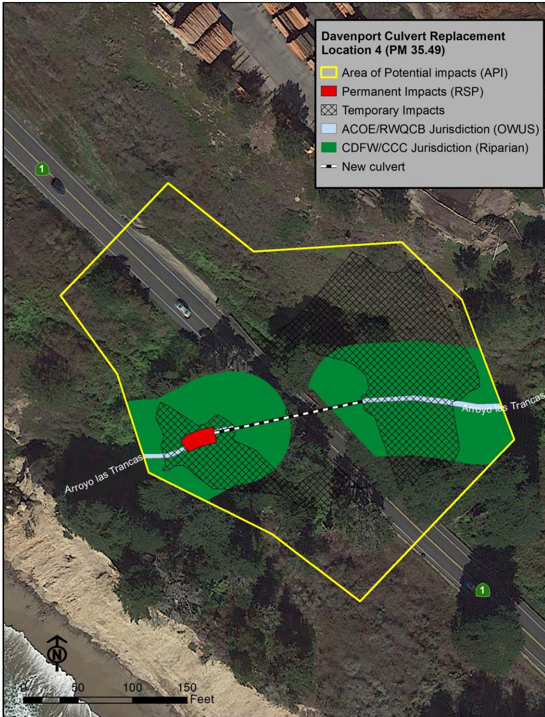
Figure 2-9 Location 4 Potential Impacts to Jurisdictional Areas
