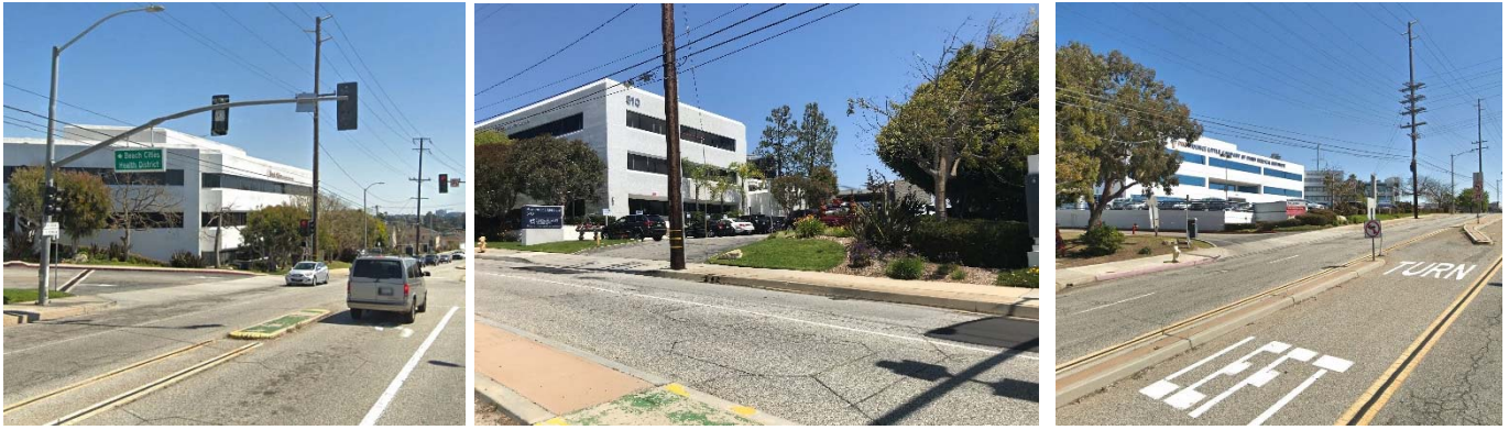
Photo 5. The main entrance to the campus (left) is located at a signalized intersection that provides for left- and right-turns into the campus. Secondary access to the Project site includes two driveways to the north (middle) and south (right) of the main entrance. These unsignalized driveways provide for right-turn only ingress/egress. These driveways also provide access to the perimeter circulation road that follows along the edge of the campus and the surface parking lots in the northwestern corner of the Project site.
