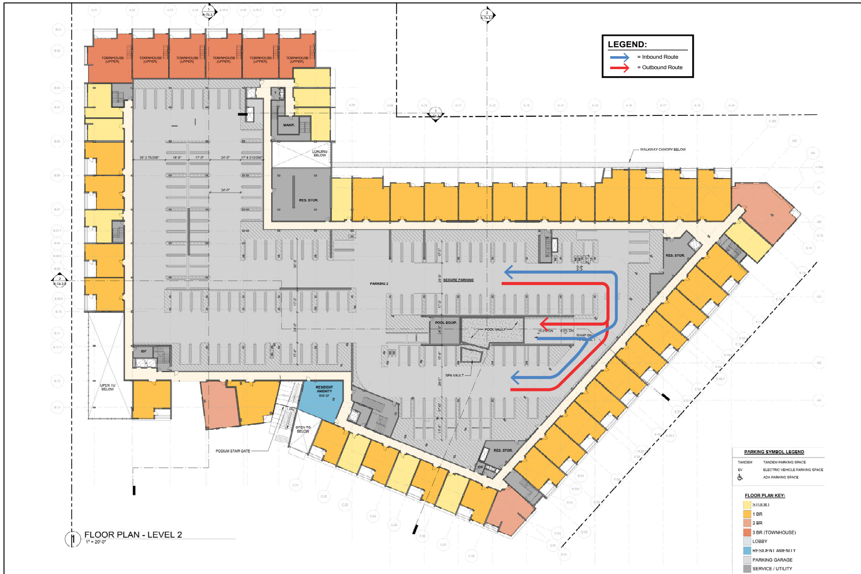
Figure 24 Residential Building Second-Level Floor Plan and Circulation
