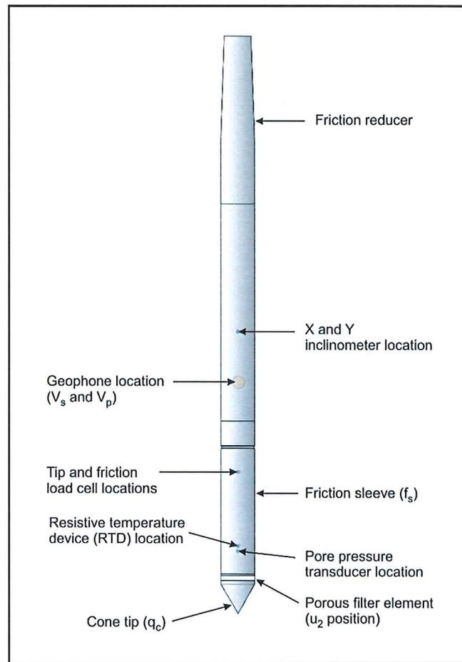
Figure CPTu. Piezocone Penetrometer (15 cm<sup>2</sup>)
