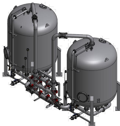
Figure 3.2. Lead/lag GAC system with 10 ft diameter vessels
