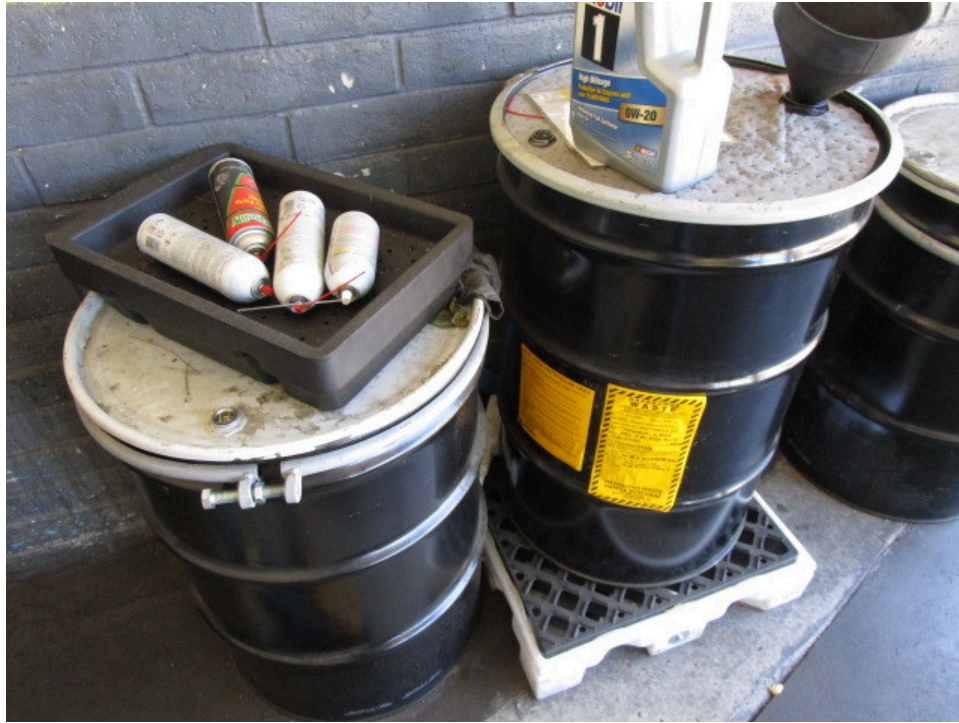
21. 55-gallon drums of used aerosol cans and used antifreeze
