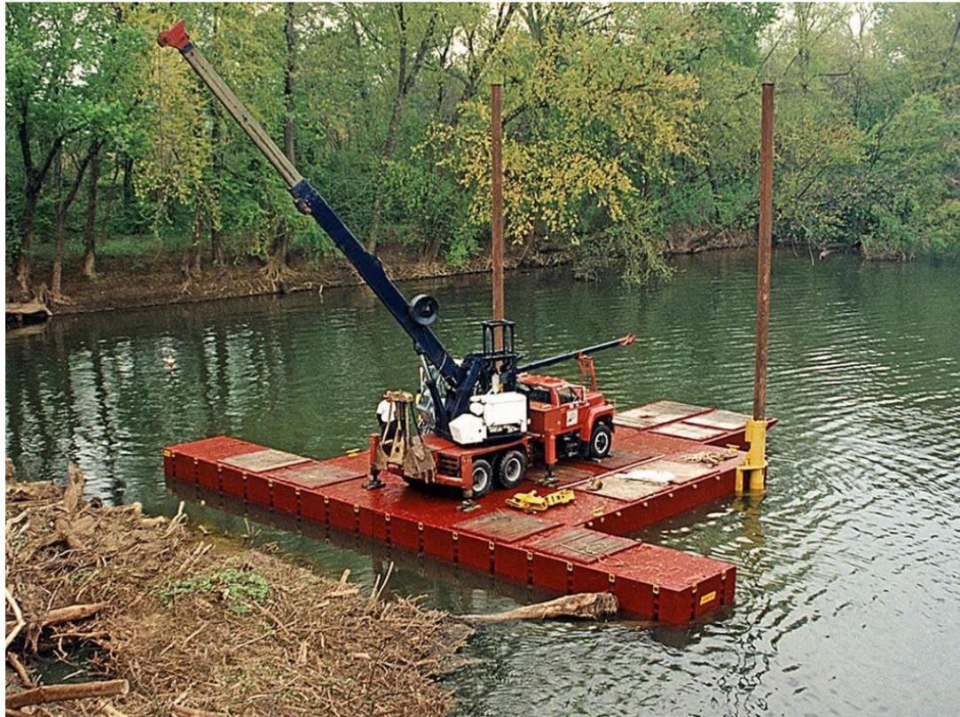
the barge would be anchored in the creek for a period of up to 12 hours, until the next high tide allowed the contractor to move it. The barge would be anchored in the channel using “spuds,” which are removable piles that would be set into the creek bed (Figure 1-11).
