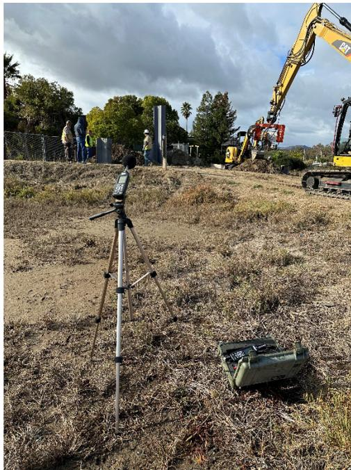
Photo 4: Noise and vibration meters at Site 2.
