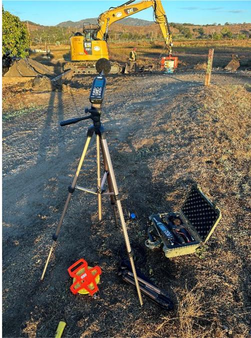
Photo 3: Noise and vibration meters at Site 1.
