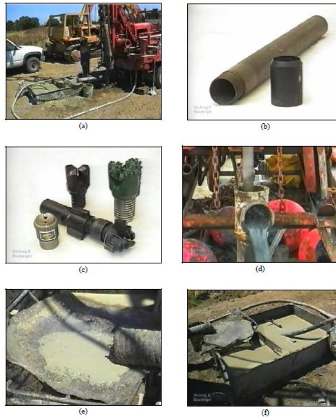
Figure 1: From FHWA Manual on Subsurface Investigations: Rotary Wash Drilling System: (a) Typical drilling configuration; (b) casing and driving shoe; (c) Diamond, drag, and roller bits; (d) Drilling fluid discharge; (e) Fluid cuttings catch screen; (f) Settling basin (mud tank).
