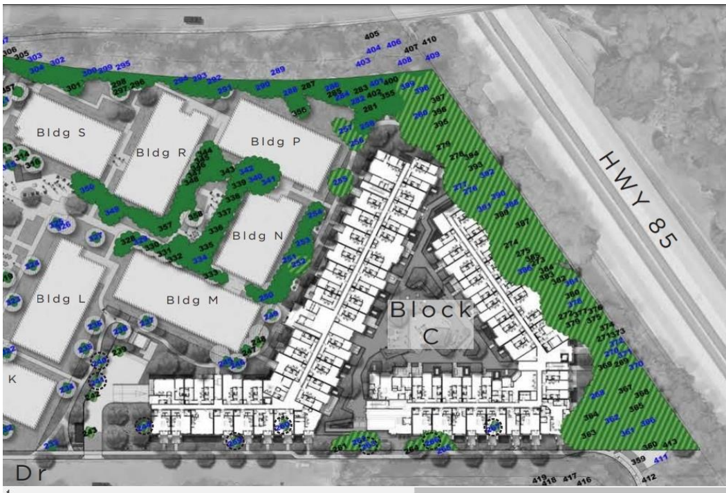
Excerpt from Drawing L.003 ‘Tree Removal Plan’ : Green hatched area shows ALL the trees along Hwy 85, on the property, are to be clear cut to make place for new buildings. Blue numbers are heritage trees, black numbers are non-heritage, and shrubs to be removed are not documented
