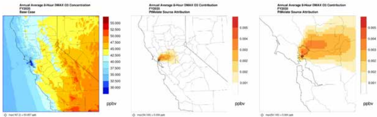
Figure 2-3. Annual Average MDA8 Ozone Concentrations from the Base Case Scenario (left) and Increases in Annual Average MDA8 Ozone Concentrations due to the Project (right) for the Annual Modeling of the 2035 Emissions Scenario
