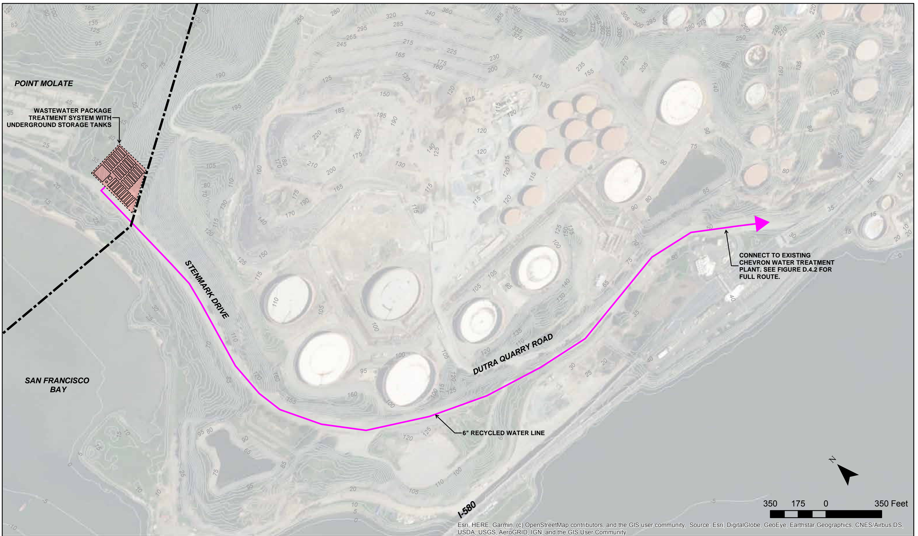
FIGURE D.4.1: OPTION B - ONSITE TREATMENT PLANT AND RECYCLED WATER ALIGNMENT POINT MOLATE DEVELOPMENT
