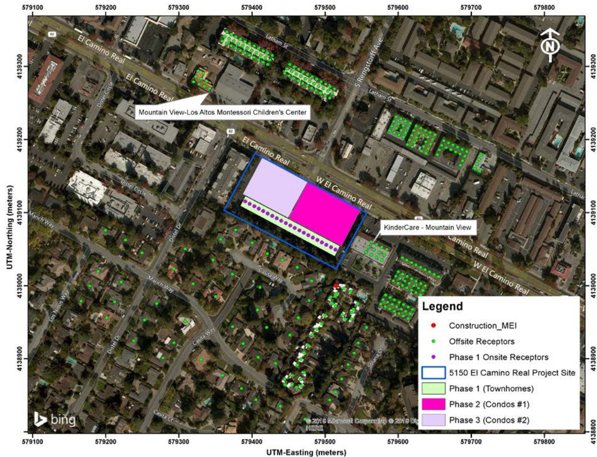
Figure 1. Project Construction Site and Locations of Off-Site Sensitive Receptors and TAC Impacts from Project Construction
