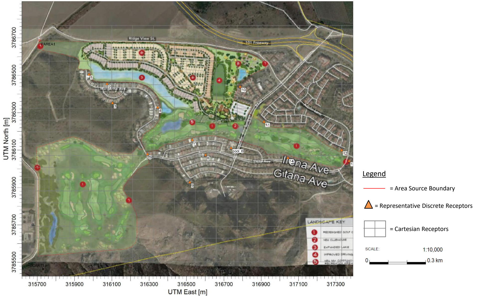
Figure 3 AERMOD Model Source and Receptor Placement
