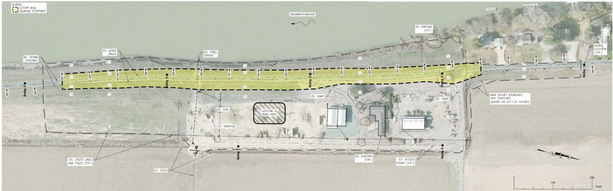
Figure 1-3. Grand Island Levee Seepage Cutoff Wall Project Area plan drawing, with cutoff wall footprint in yellow.
