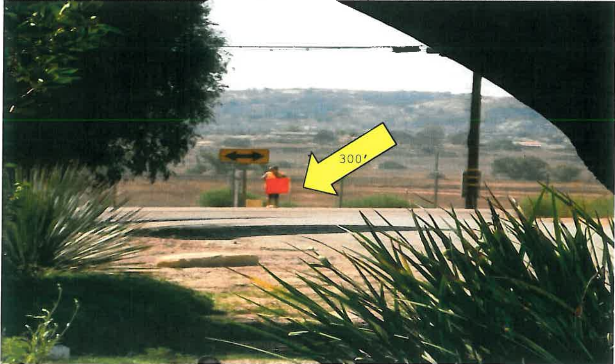
Looking South at northbound traffic on Montecito Way 300' feet from Driveway #3, 8' feet from edge of pavement, from a height of 3.5' feet to a point 4.25' foot high on Montecito Way in the center of the northbound travel lane (Zoomed In)
