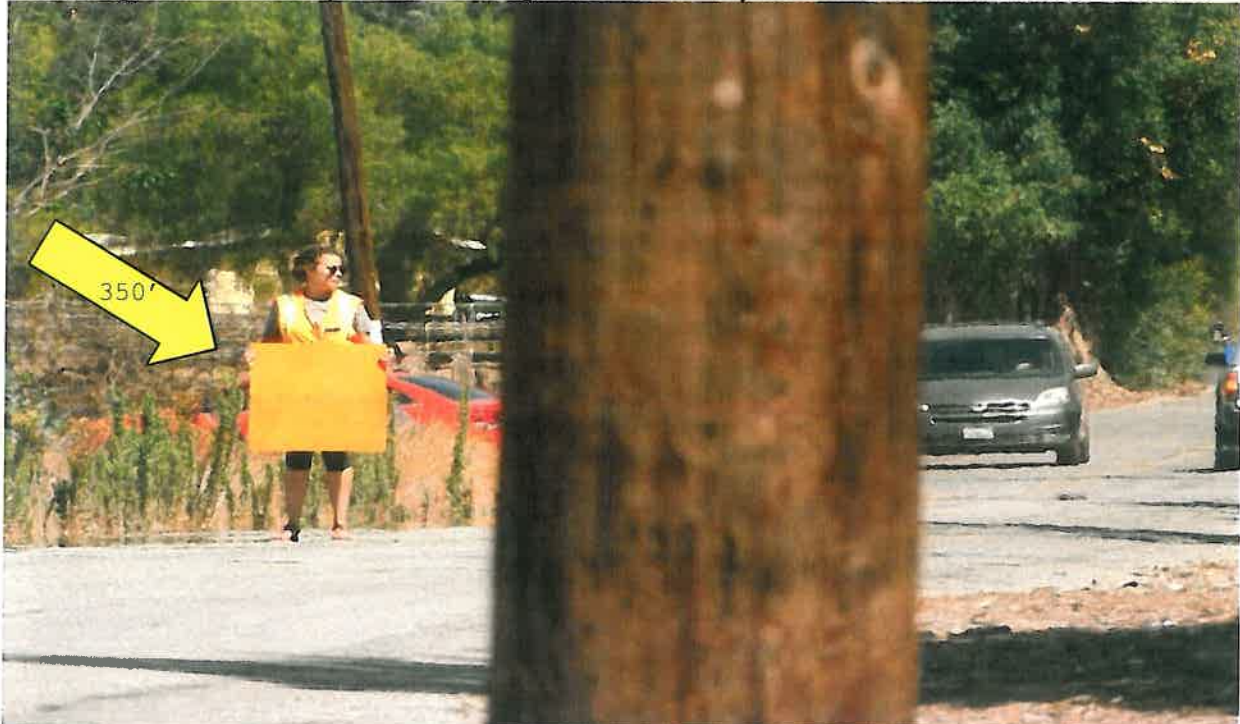
Looking North at southbound traffic on Montecito Way 350' feet from Driveway 2, 8' feet from edge of pavement, from a height of 3.5' feet to a point 4.25' foot high on Montecito Way in the center of the southbound travel lane (Zoomed In)
