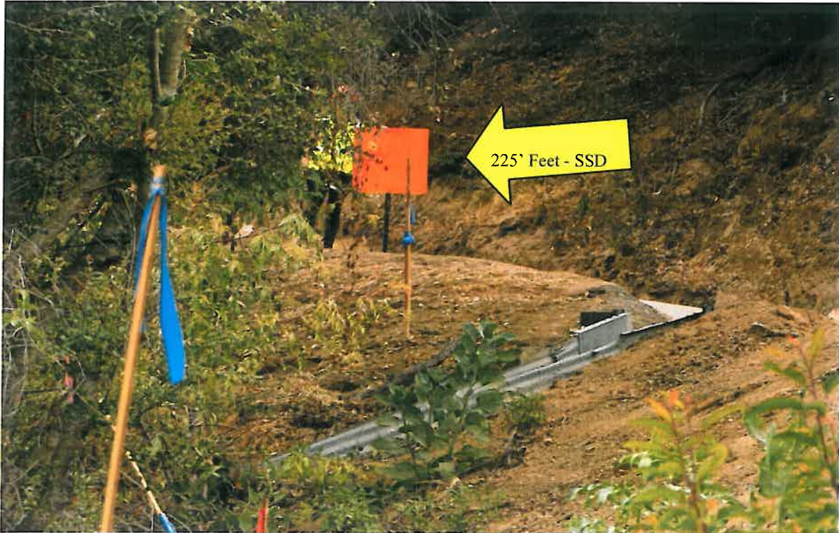
Looking East on Highland Valley Road from the projects driveway to provide 225' Feet Stopping Sight Distance (SSD). (Zoomed In)
