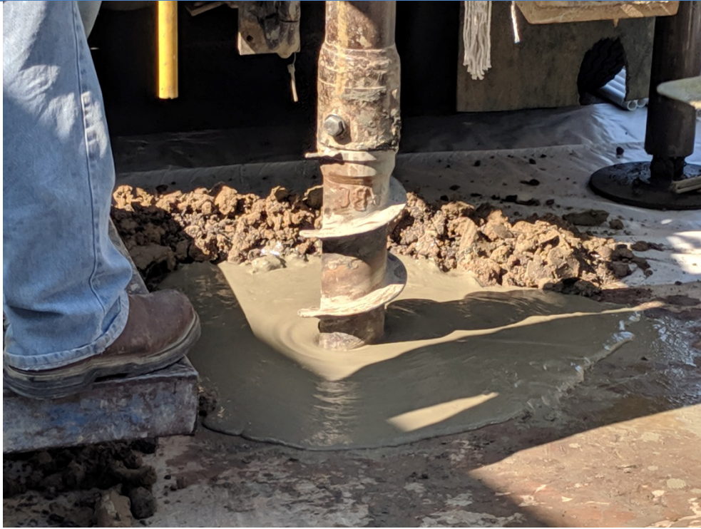
PHOTO 3: Drilling within the saturated zone (B1) (7/16/19).
