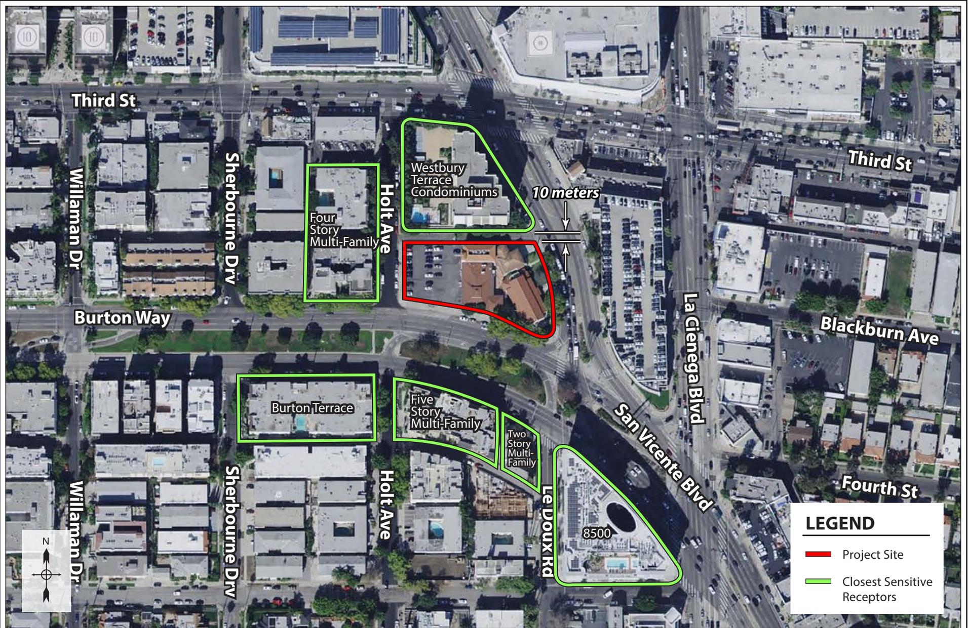
The closest receptor distance on the mass rate LST look-up tables is 25 meters. Projects with boundaries located closer than 25 meters to the nearest receptor should use the LSTs for receptors located at 25 meters.
