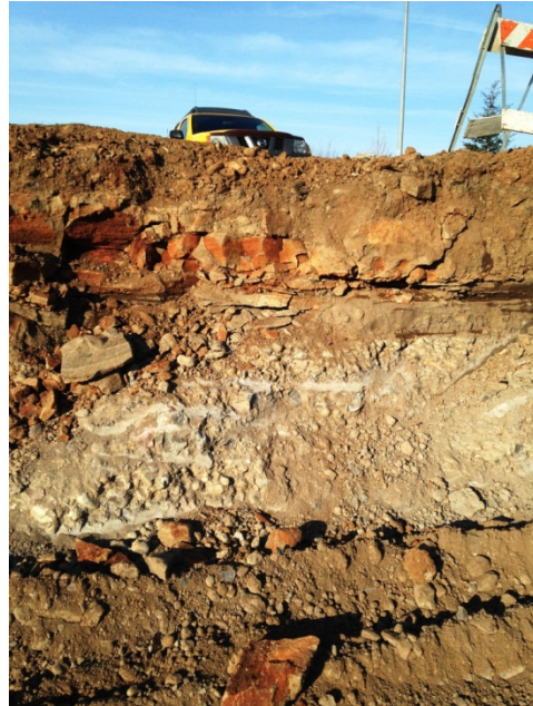
Photo 6: 6 foot thick section of sandstone and conglomerate within storm drain trench exposure at the end the existing paved Doe Mill Road (Section 226). Per the trenching contractor, very hard lahar underlies the conglomerate at the bottom of the photo.
