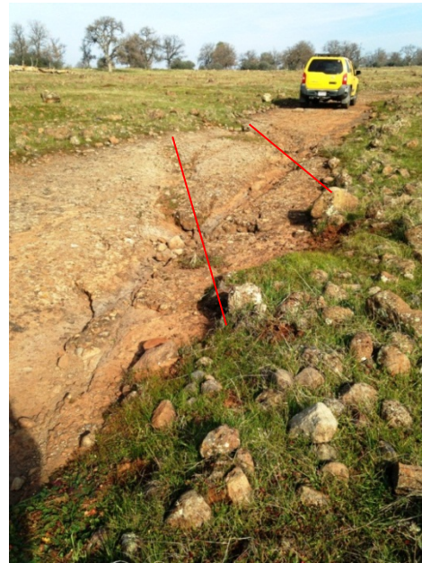
Photo 4: Doe Mill Road at Section 232. Lahar has been exposed by removing 2 to 5 inches of soil. Red lines demark two NNE trending, near vertical fractures within the lahar that are common to the site and vicinity.
