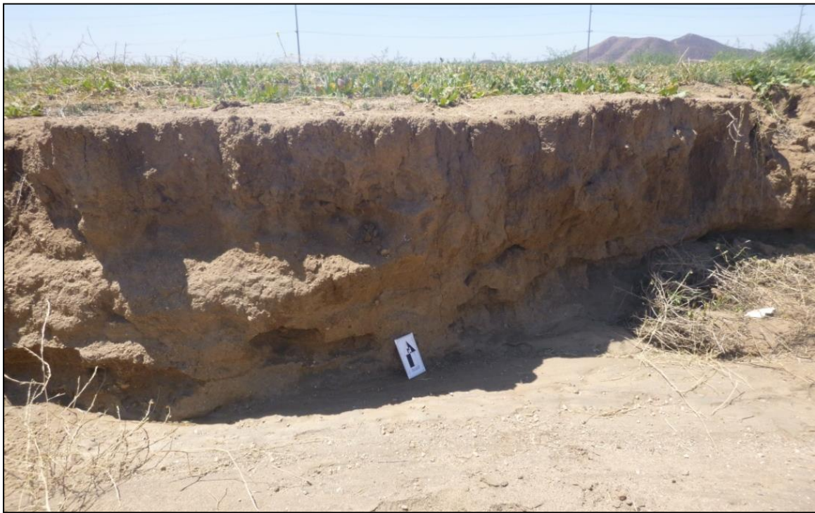
Figure 6-4 Quaternary older alluvial fan deposits in the Project area, composed of poorly consolidated, tan to brown, coarse granitic gravel, sand, and silt. Poorly exposed below approximately 2 – 4 feet of soil development, view to the south.
