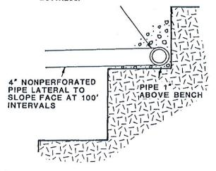
\* GRADED FILTER MATERIAL TO CONFORM TO STATE OF CALIFORNIA DEPT. OF PUBLIC WORKS STANDARD SPECIFICATIONS FOR CLASS 2 PERMEABLE MATERIAL
