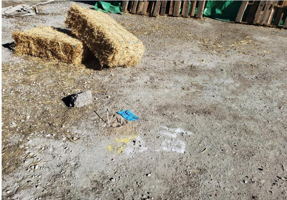
**Photograph 5:** Vapor probes installed and at Boring B4 at approximately 5 and 10 feet below ground surface.
