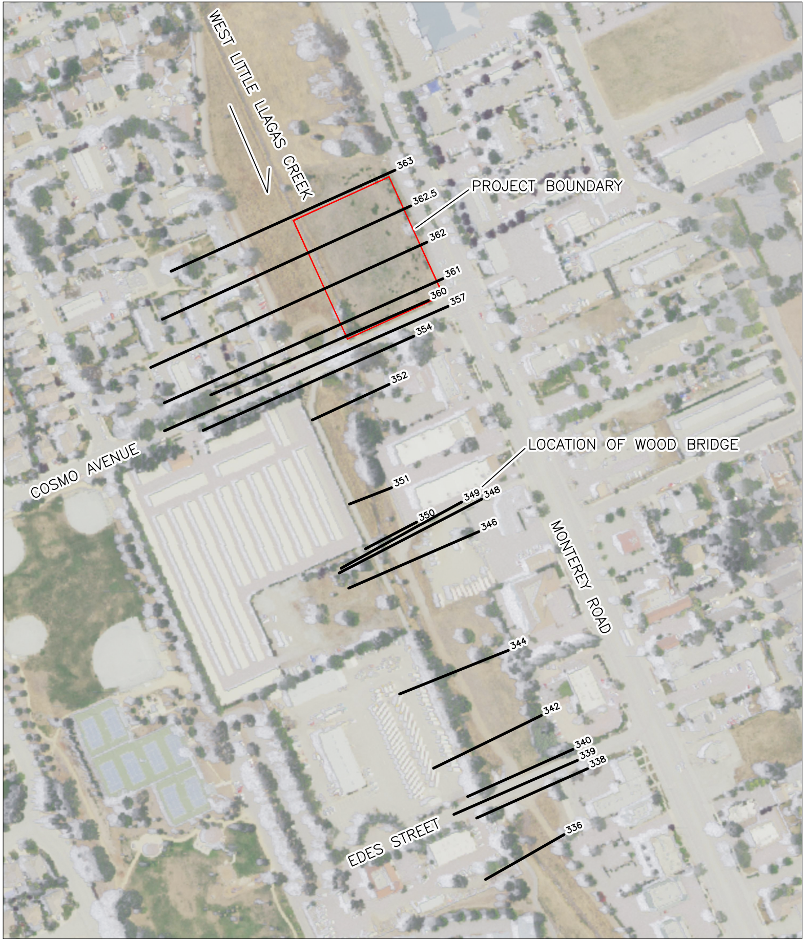
Figure 2. Revised hydraulic model cross sections, West Little Llagas Creek at Voices School site, City of Morgan Hill.
