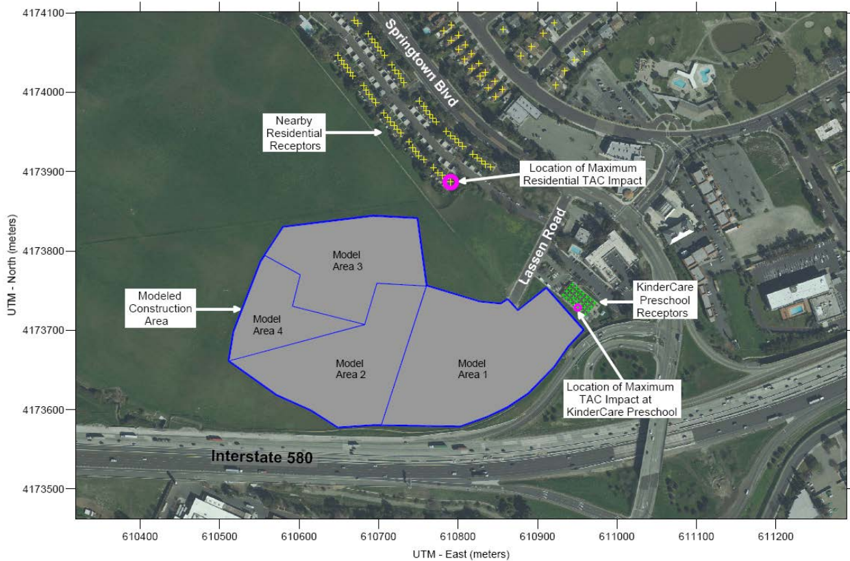
Figure 2. Project Construction Site, Area Sources Used for Modeling, and Locations of Off-Site Sensitive Receptors and Maximum TAC and PM 2.5 Impacts
