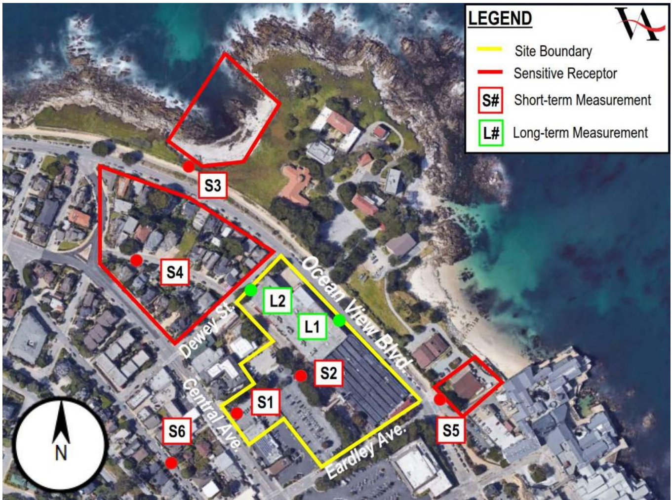
Figure 2 Aerial View of Project Site Showing Measurement Locations
