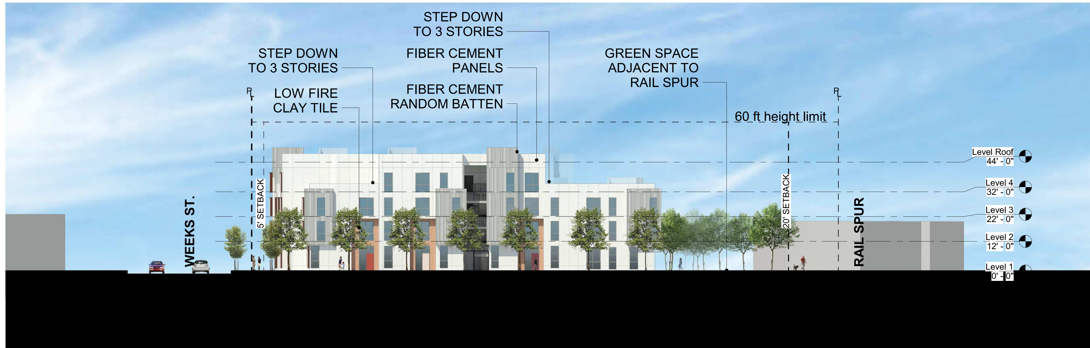
① EAST ELEVATION (RAIL SPUR CONNECTION) 1" = 20'-0"
