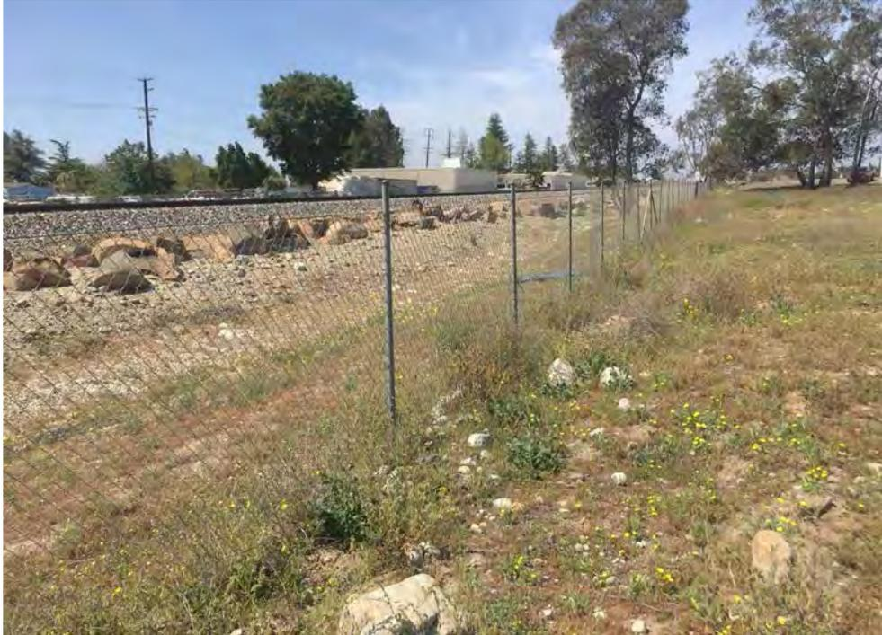
Photo 9. Approximately three-foot wide manmade ditch along railroad tracks (Ditch 2) within 100-foot buffer south of project site boundary and north of East 8<sup>th</sup> Street. (Ditch 2 is shown on the left side of the fence in the above photo). Ditch 2 displayed no evidence of drainage patterns, an OHWM, and/or streambed and appeared to be a ditch created in uplands to for localized runoff-conveyance purposes.
