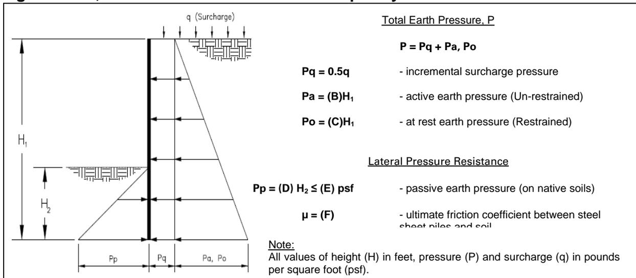
The provided pressures assume no hydrostatic pressures. If hydrostatic pressures are allowed to build up, the incremental earth pressures below the ground-water level should be reduced by 50 percent and added to hydrostatic pressure for total lateral pressure.
