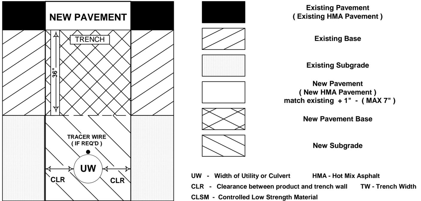
STRUCTURE BACKFILL SHALL CONFORM TO SECTION 19 - 3.06 OF THE STANDARD SPECIFICATIONS
