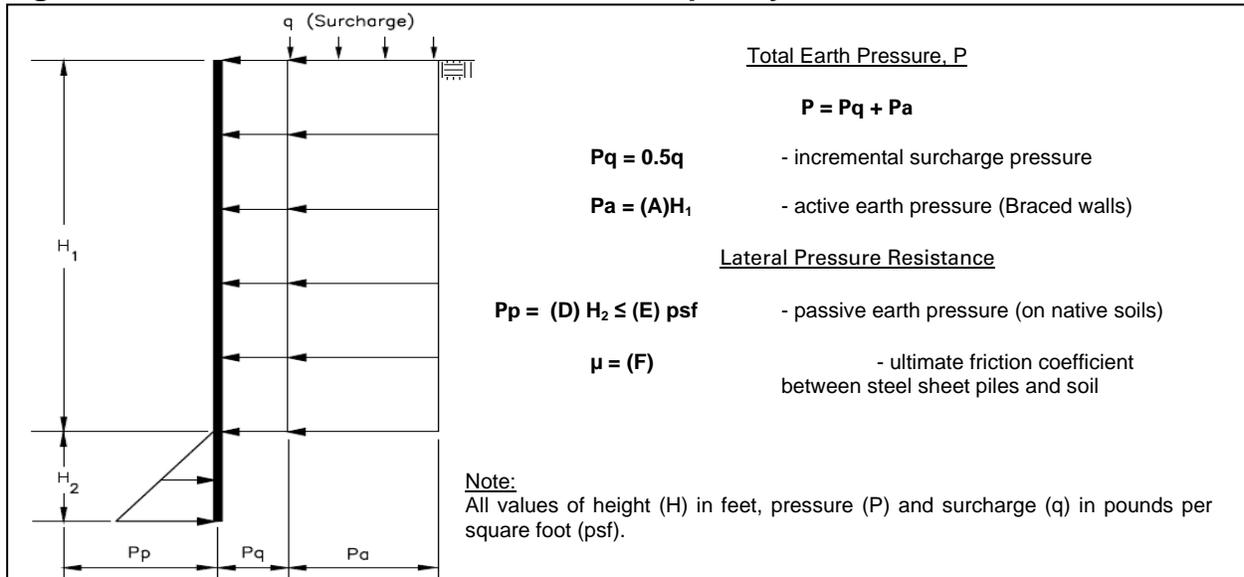
Unrestrained (cantilever) design of cantilever shoring consisting of soldier piles spaced at least two diameters on-center or sheet piles, can be based on Figure No. 4, *Lateral Earth Pressures on Temporary Cantilever Wall*.
