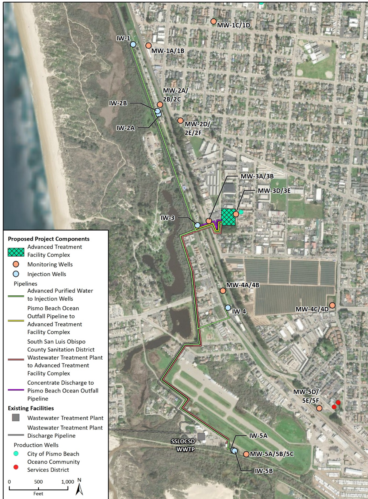
Figure 2-4 Project Components with Known Locations – Focused Extent
