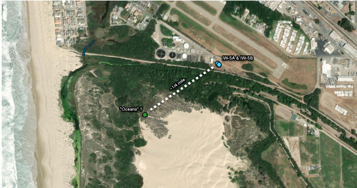
Figure 1. Proposed injection wells (IW-5A & IW-5B) and plugged and abandoned oil well ("Oceano" 1). To view information and locations for oil and gas wells visit https://www.conservation.ca.gov/calgem/Pages/WellFinder.aspx
