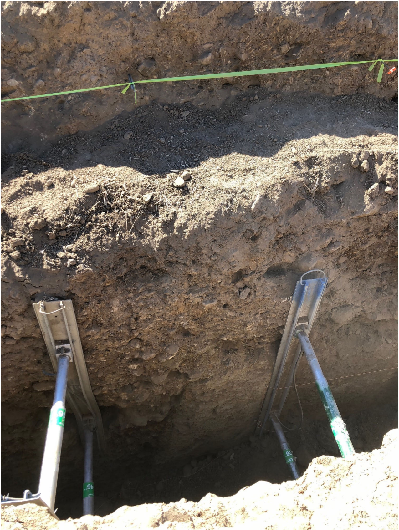
This easterly view spans over abrupt contact between Station 35 to Station 40. Green ribbon is placed along base of A-Horizon residual soil (unit 1a). No change in thickness of Unit 1a or underlying Unit 1b over this contact (Photo credit: CSH, 2021)
