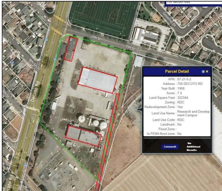
Figure 2. Aerial view of industrial plant at 700 Decoto Road, outlined in green, facing north. Three age-eligible buildings and a small branch of the SPRR spur are outlined in red (administrative office building to the northwest, compressed gas plant at center, air separation plant/compressor house to the south, and a small branch of the SPRR spur to the east). Source: Union City Property Information Map, 2019; edited by ICF, 2019.
