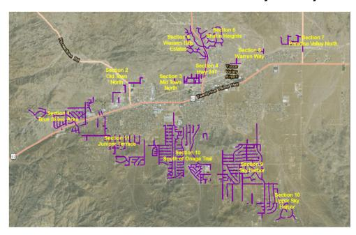
The Hi-Desert Water District (HDWD) is proposing to construct approximately 64 miles of PVC sewer pipeline, 1,300 manholes and three lift stations facilities in various areas of its service territory over the next 10 years for the purpose of decreasing the reliance on septic systems in their service territory.
