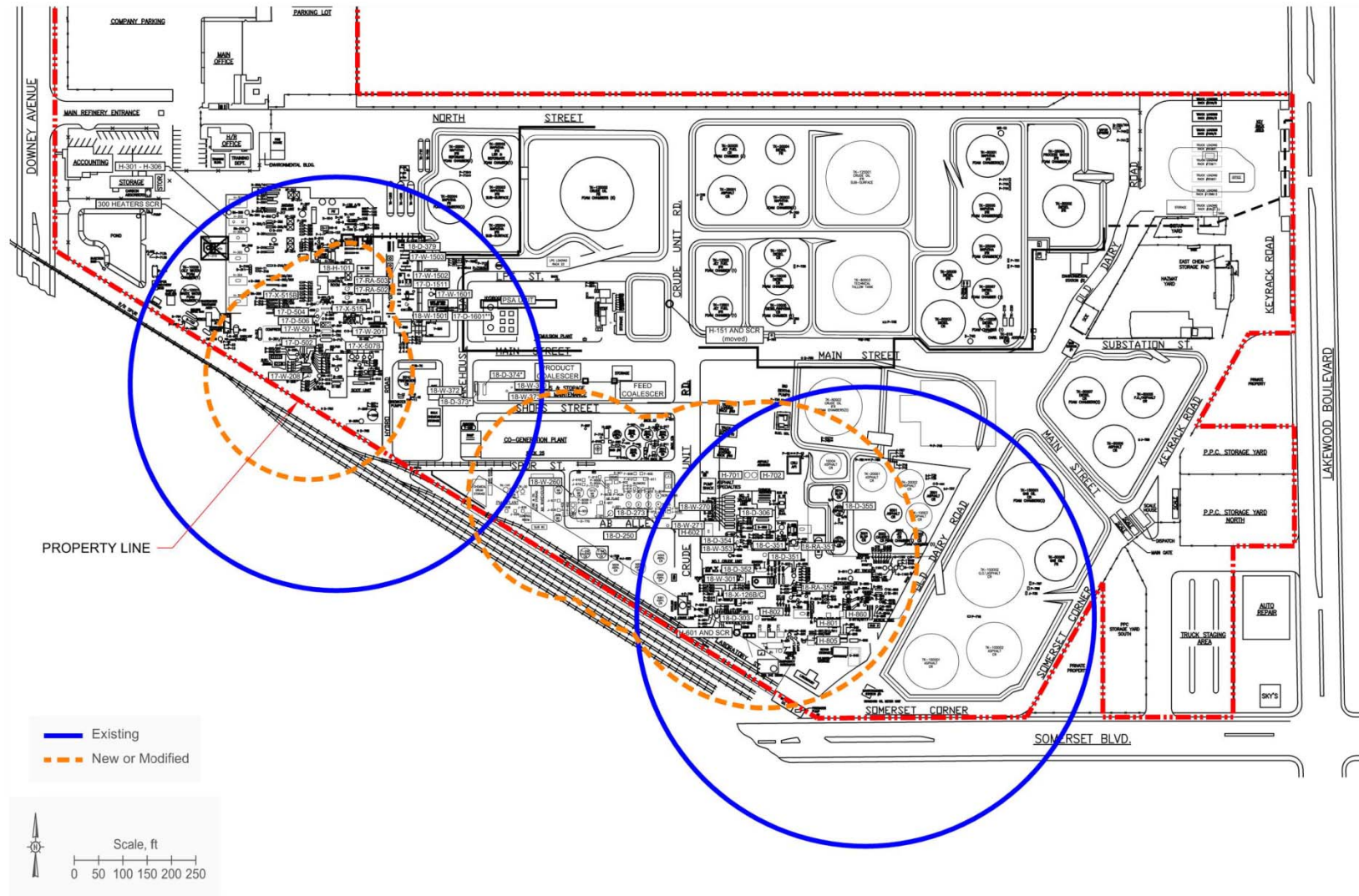
Figure C-4 Toxic Composite Vulnerability Zone for Existing and New/Modified Equipment
