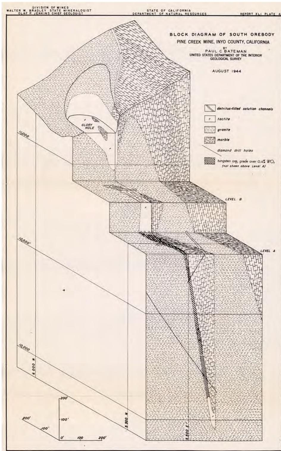
**Figure 13.** South Orebody showing mining levels and glory hole (State of California, Department of Natural Resources, Report XLI, Plate 43, *Block Diagram of South Orebody, Pine Creek Mine Inyo County, California*, August 1944. California Geological Survey Library, Sacramento) (SC, DNR 1944a).
