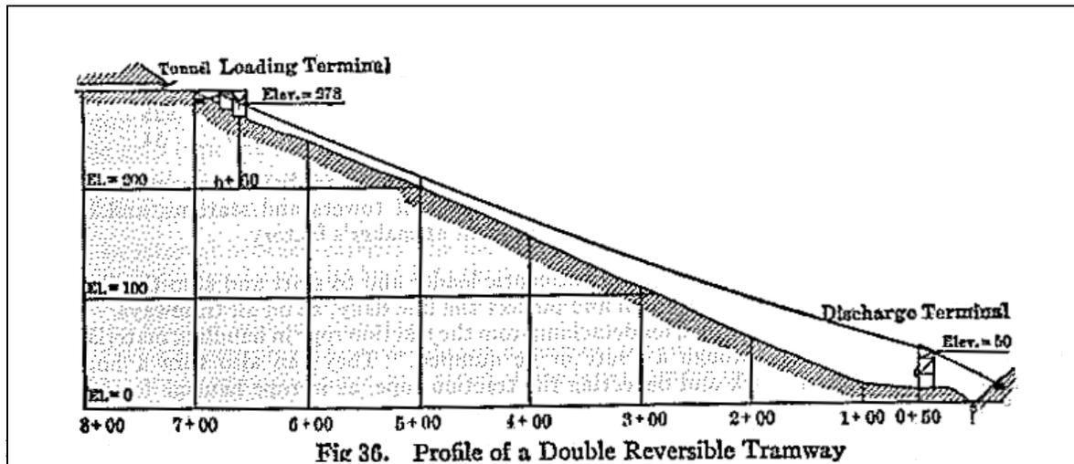
**Figure 37.** Diagram of Double Reversible Tramway Used for Mining Ores (Peele 1927:1784).
