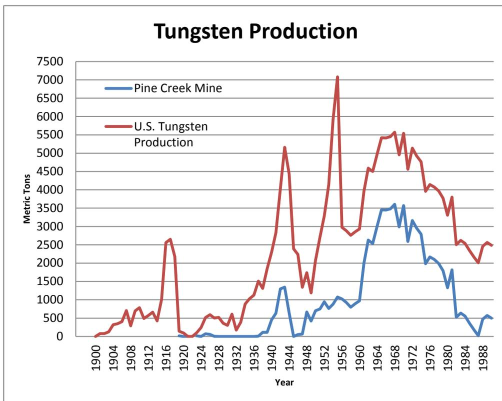
**Figure 20.** Tungsten Production (Kurtak 1998:198-1999; USGS 2012). USGS provided information for Tungsten production in the United States in two categories “Primary Production” and “Secondary Production,” which were added together to create a total production number used for this table. Pine Creek Mine production information furnished by Kurtak was listed in Units of  $WO_3$ , which was converted into metric tons for use in this table.
