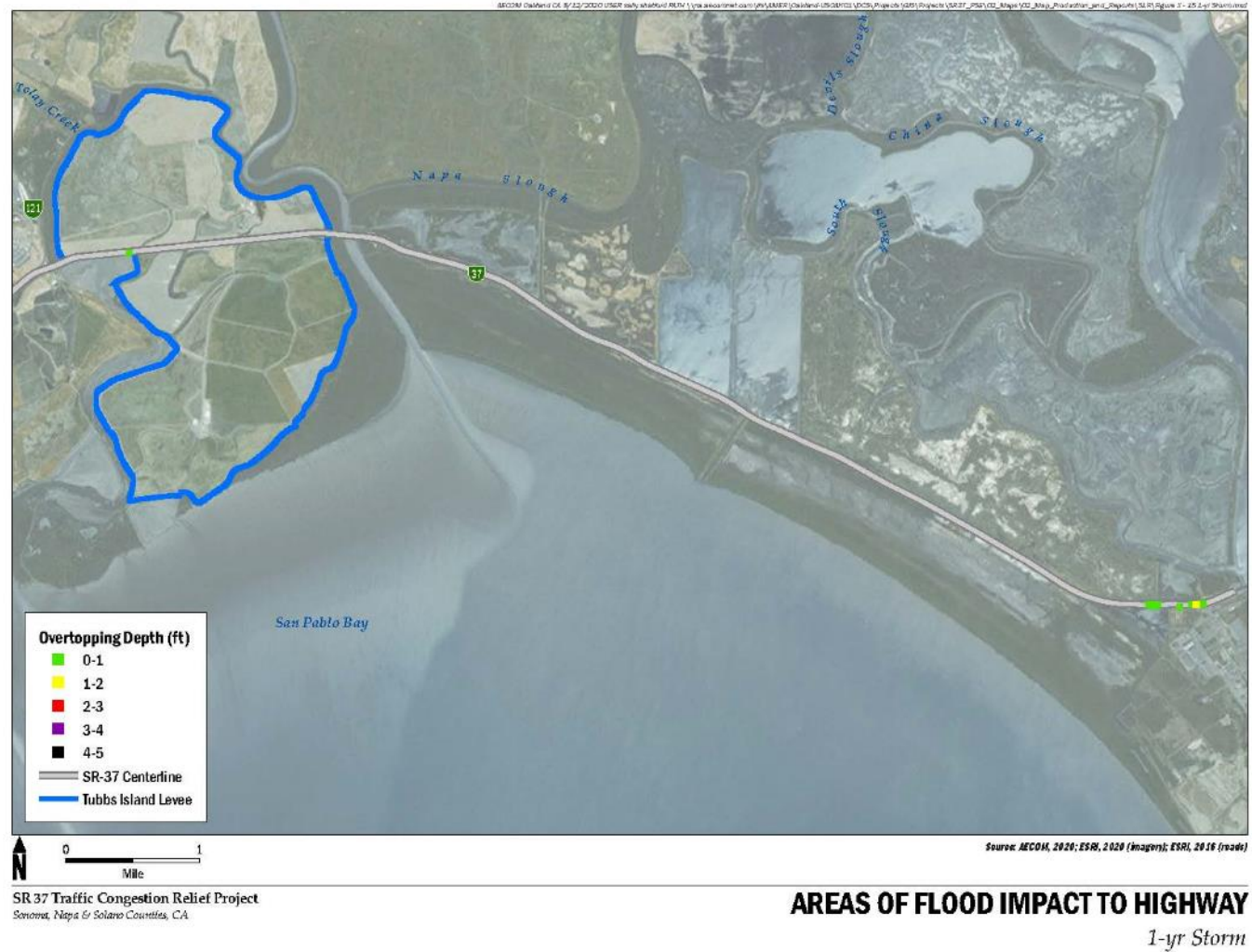
Figure 3-9 Areas of Flood Impact to Highway Under Existing Conditions with a 1-Year Storm Scenario
