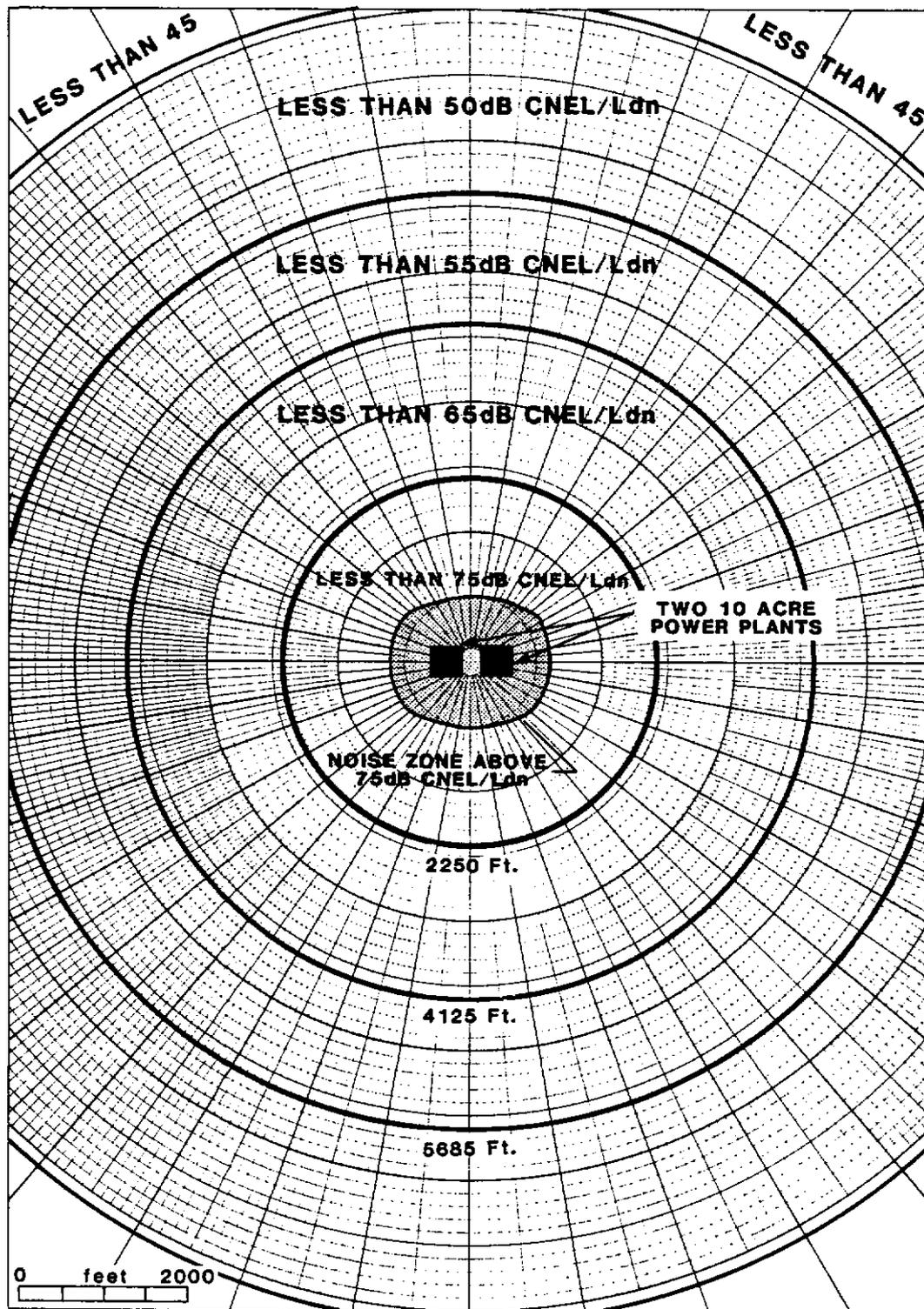
NOTE: This figure indicates the distance for compliance with CNEL/LDN Noise Standards.
