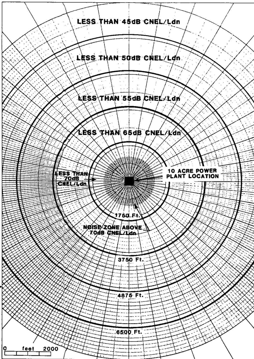
NOTE: This figure indicates the distance required for compliance with CNEL/LDN Noise Standards.
