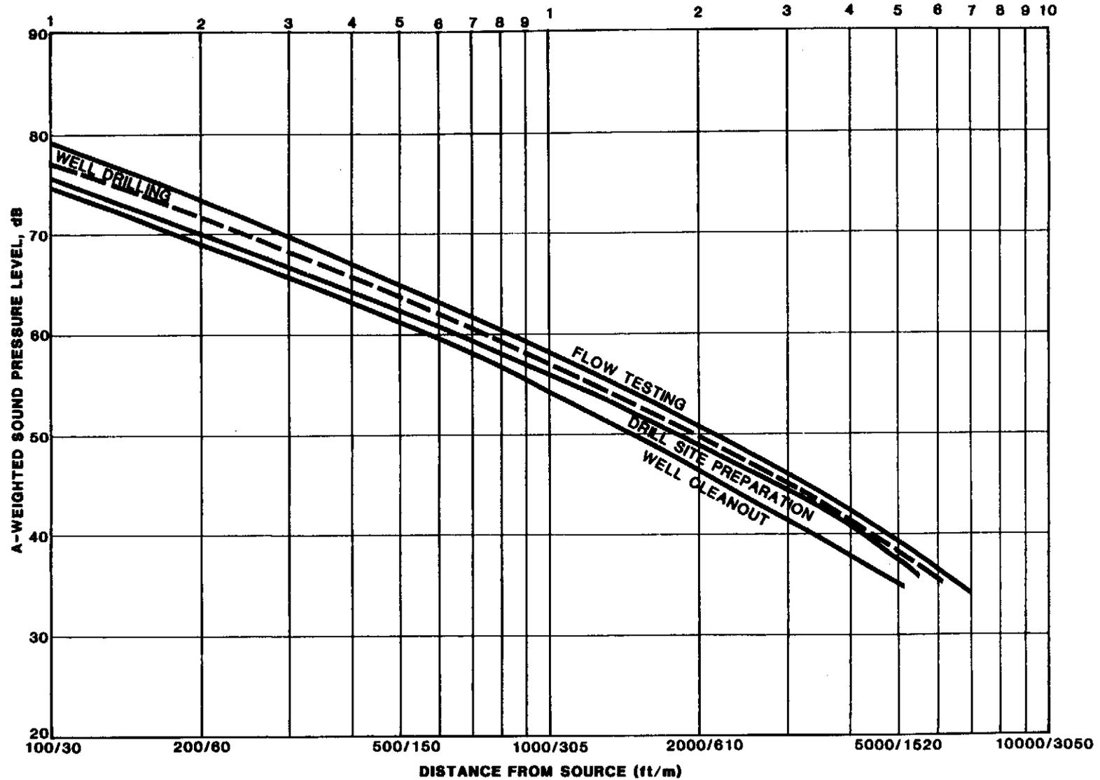
A-Weighted Sound Pressure Levels as a Function of Distance from Noise Source for Preoperational Phases of a Geothermal Power Generation Project
