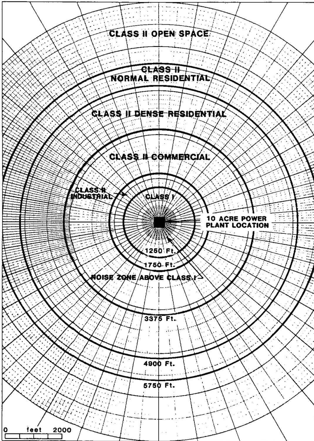
NOTE: This figure indicates the distances required for compliance with the County's standards for Initial Geothermal Development.
