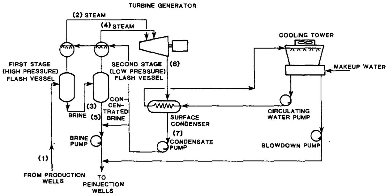
Schematic of a Two-Stage Flashed Steam Energy Conversion Process
