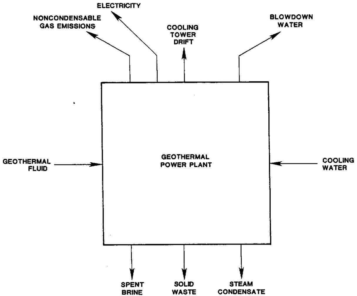
Simplified Overview of a Typical Power Plant Operation
