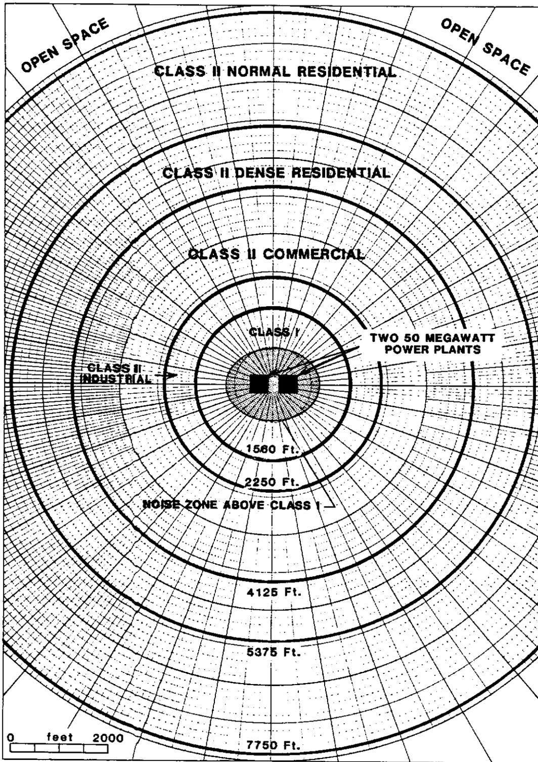
NOTE: This figure indicates the distance required for compliance with the County's standards for Initial Geothermal Development.
