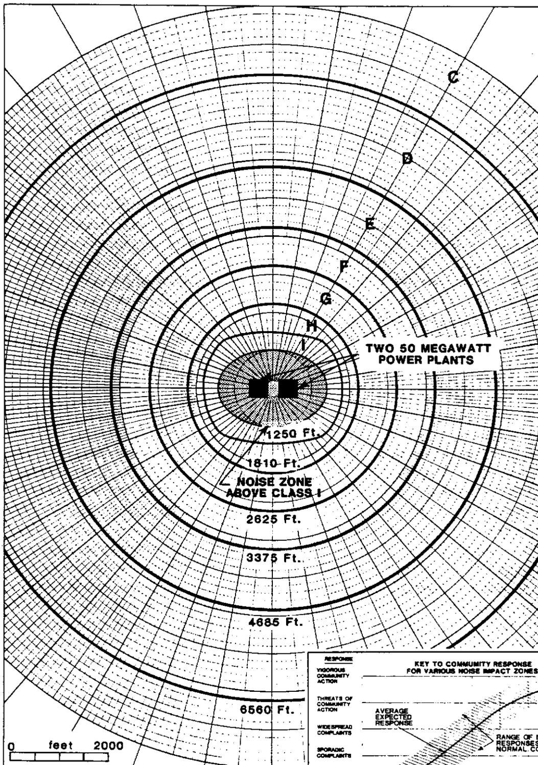
NOTE: This figure indicates the distance required for compliance with the County's Noise Element.
