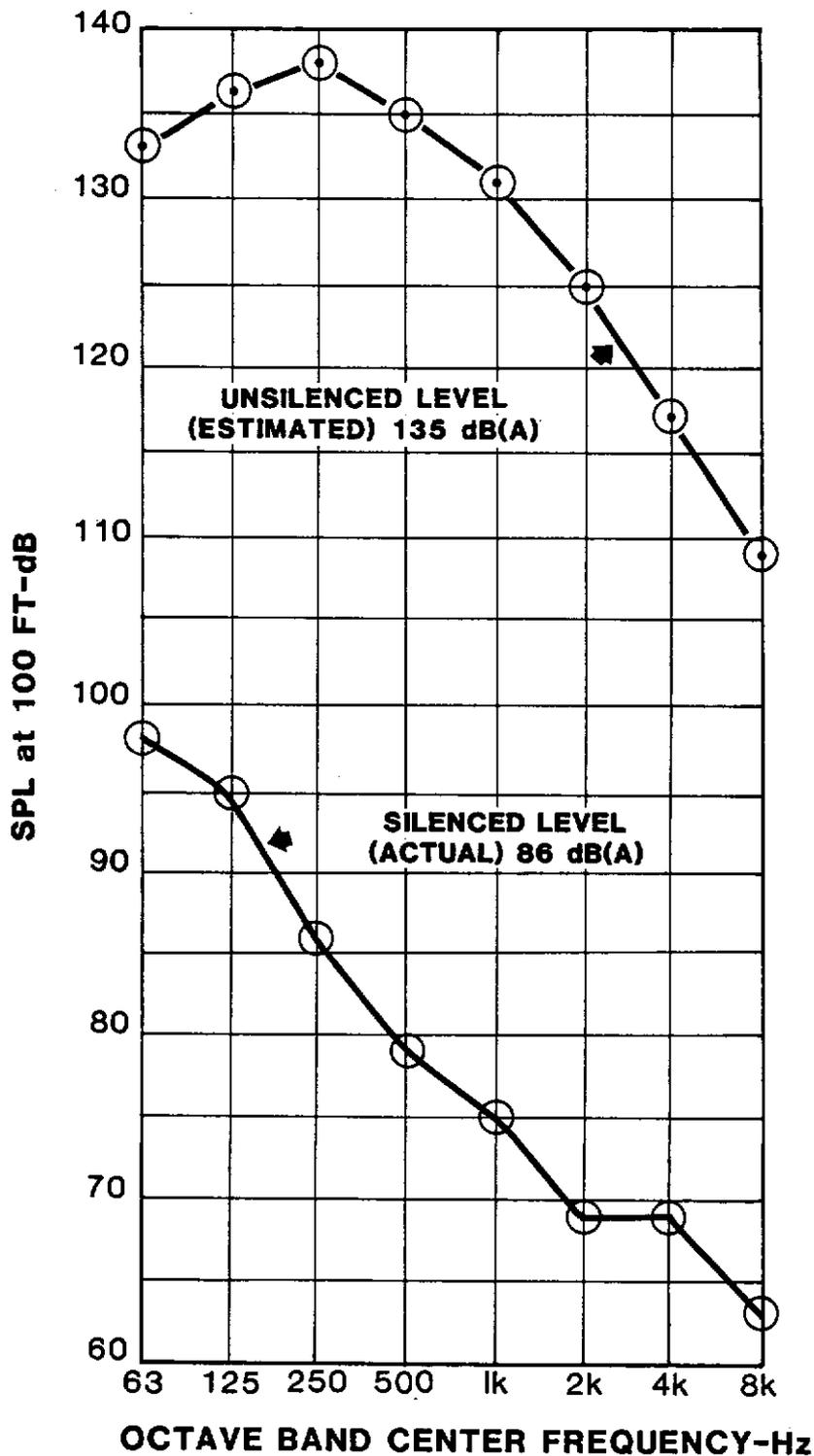
Example of Noise Reduction from a Portable Steam Blow-Off Silencer
