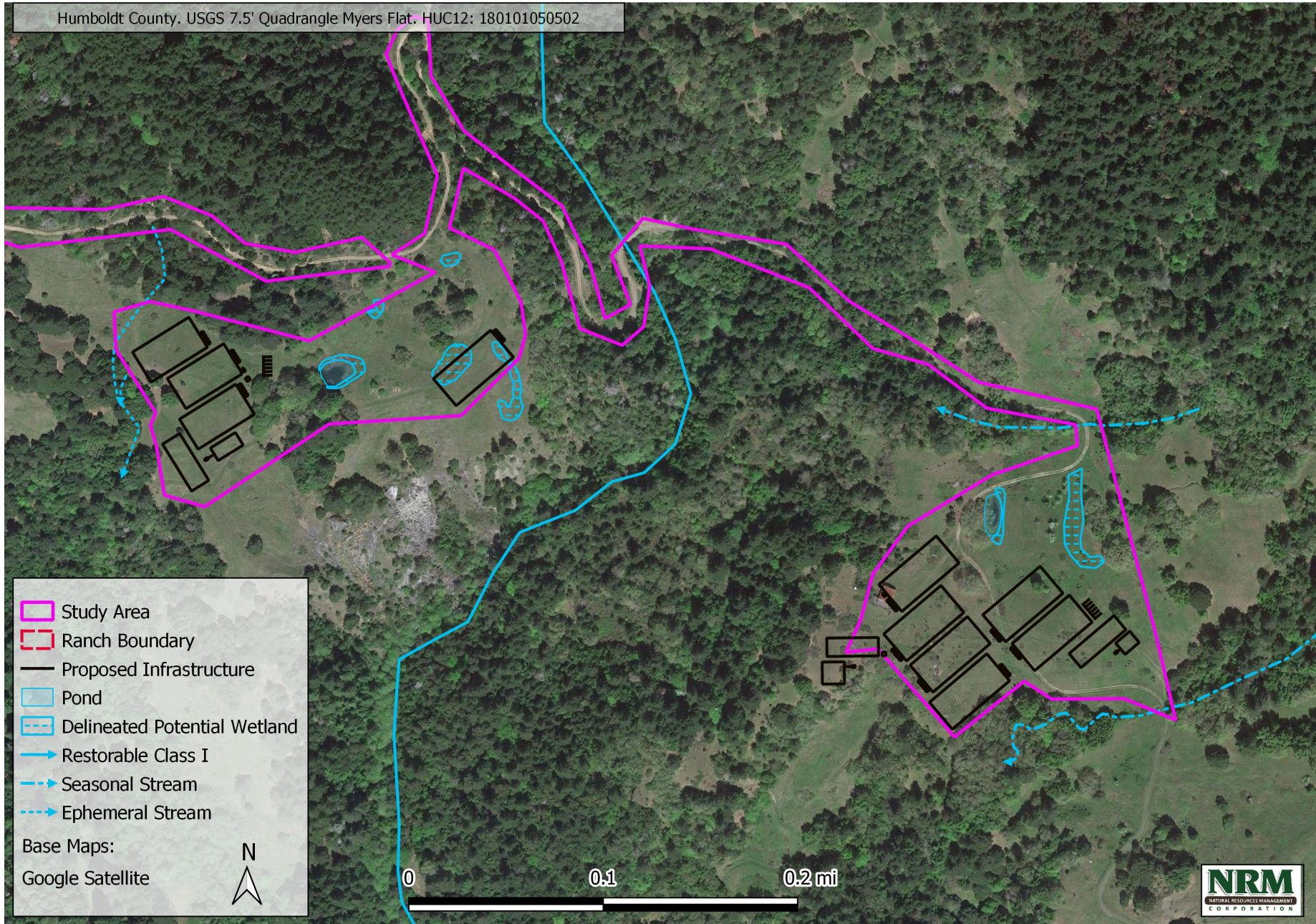
Figure 6. Relevant Hydrological Features 2 of 2. Note infrastructure layout has changed since this map was made.
