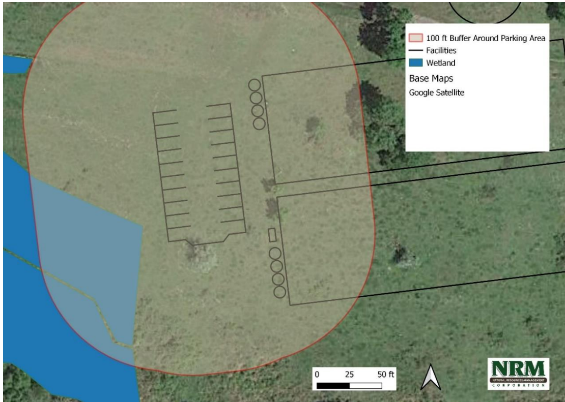
Figure 44. Wetland Impacts at Facility #9. Direct impacts to 0.239 acres of wetland are shown in red. An additional 0.047 acres of wetland lies within the 100ft buffer of the greenhouse. The parking area at Facilities #1 and #2 will not directly impact wetlands but will be within 100 feet of 0.18 acres of wetland
