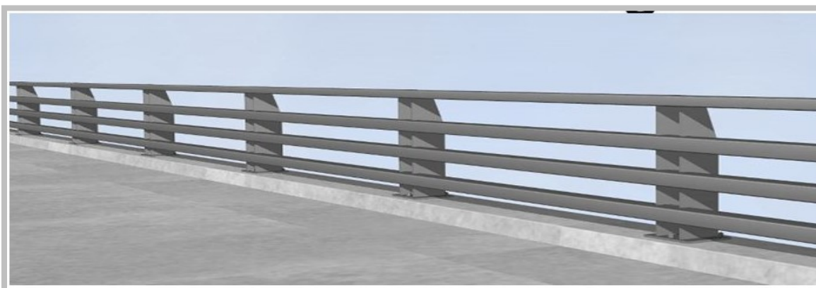
Appx. Figure 7. Bridge Railing Type California ST-75
