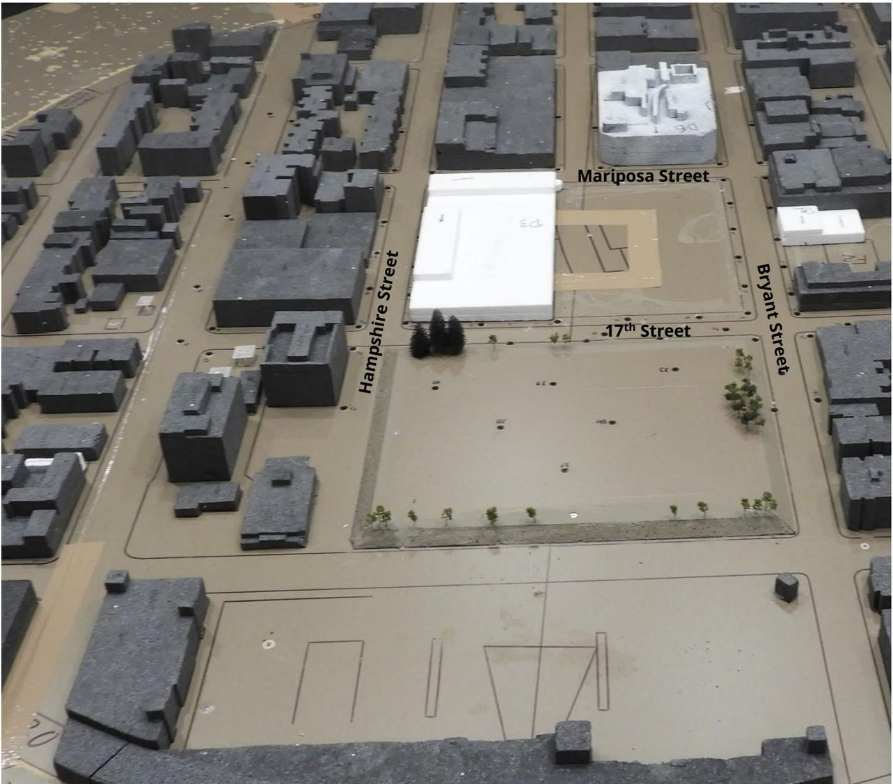
Image 2A: Wind Tunnel Study Model – Existing Configuration
