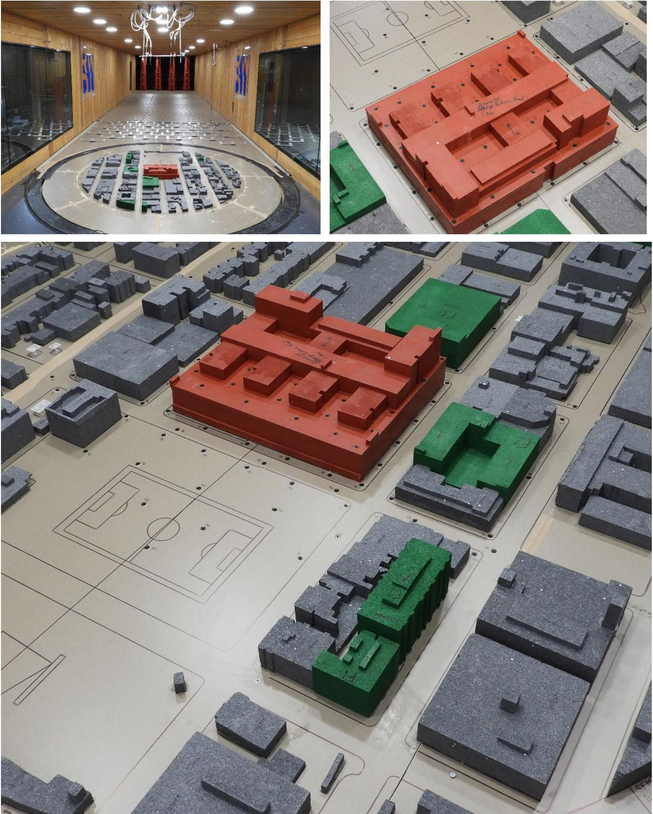
Image 2C: Wind Tunnel Study Model – Project + Cumulative Configuration
