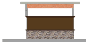
4 TRASH ENCLOSURE LEFT ELEVATION TYPE B 1/4" = 1'-0"
