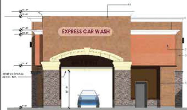
2 CAR WASH EXIT ELEVATION 1/4" = 1'-0"
