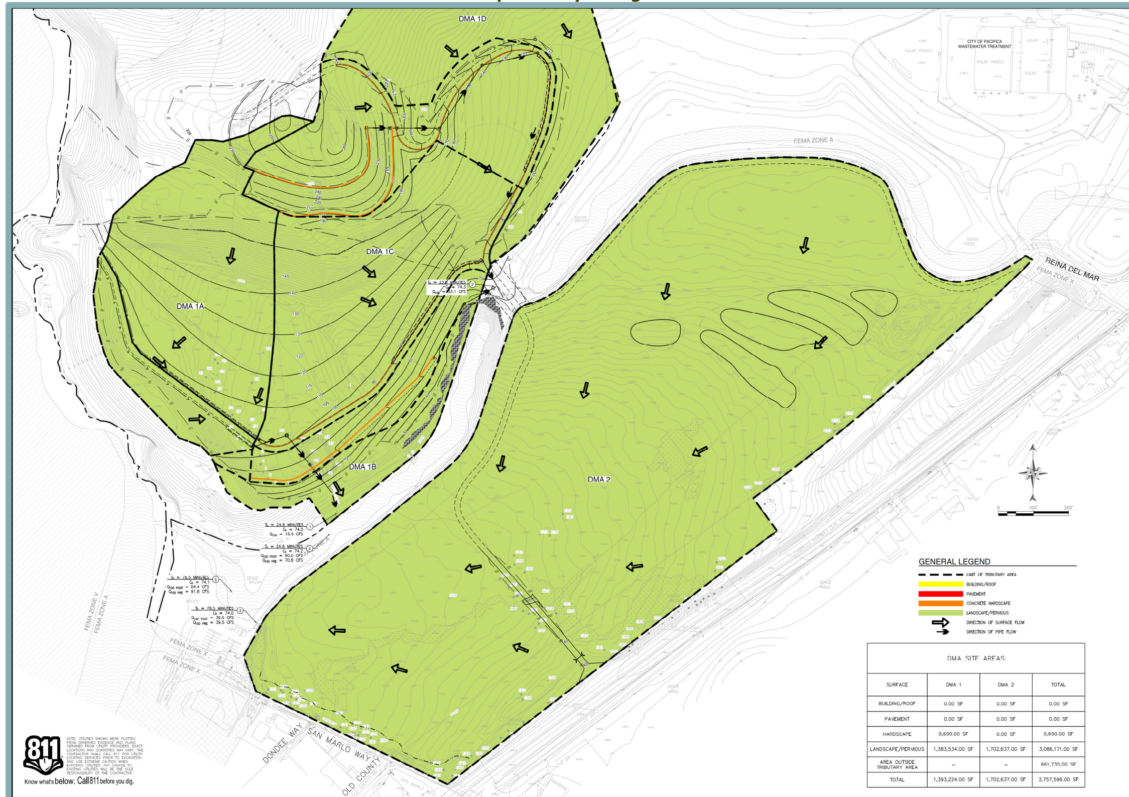
Figure 4.6-4 Post Development Hydrologic Conditions
