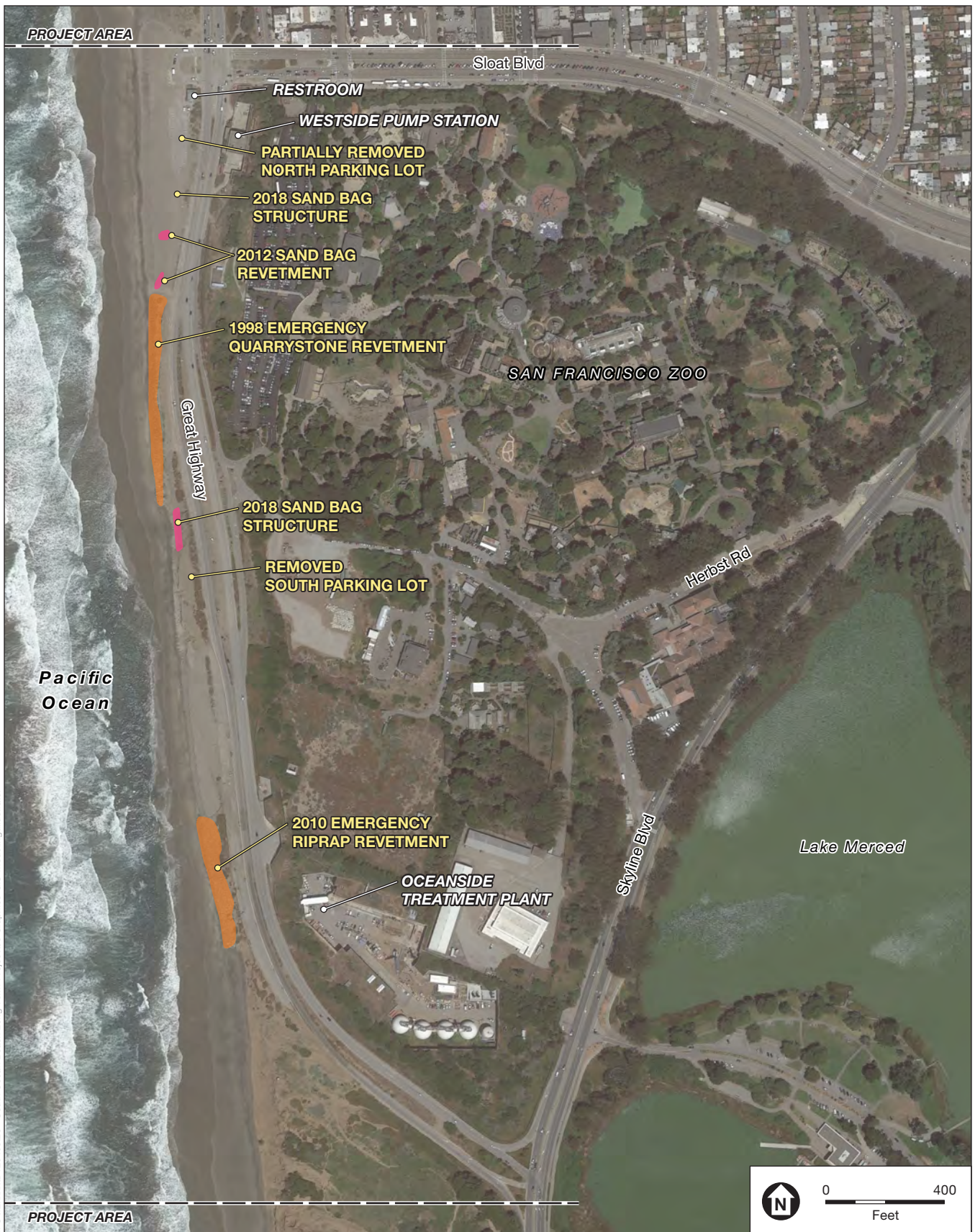
Figure 1-5 Sandbag and Rock Revetments along South Ocean Beach
