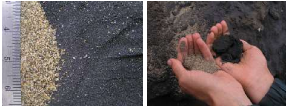
Figure 1b. Ocean beach berm sand (granitic lithology) and heavy mineral sand (magnetite lag), inch scale. Thick magnetite deposits are found only on beachfaces, and are absent in dunes, except as thin, local laminations.
