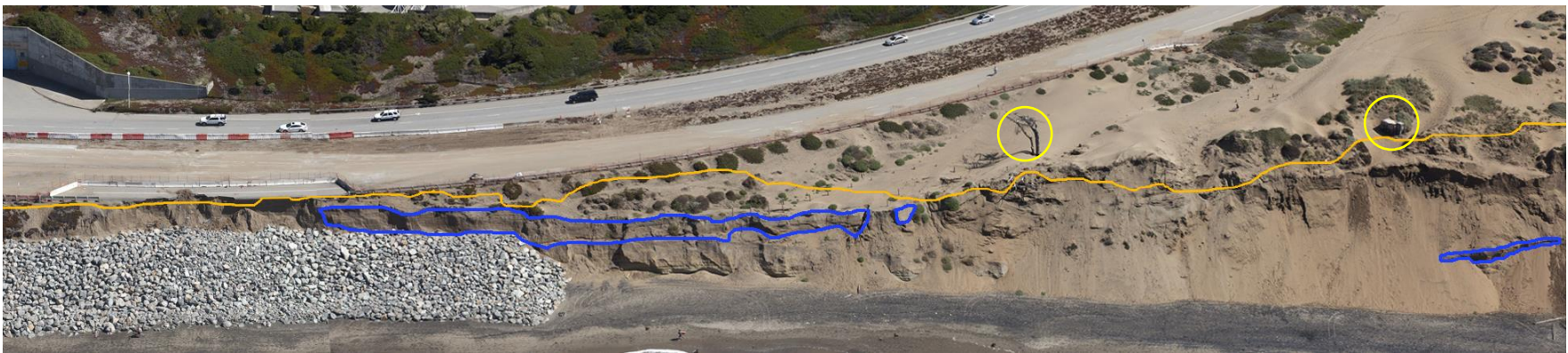
CCR imagery from September 25, 2010 shows continued coastal erosion, the addition of the rock revetment to protect critical infrastructure from erosion, and a further reduction in available bank swallow habitat. The approximate 2019 bluff line is shown in orange.
