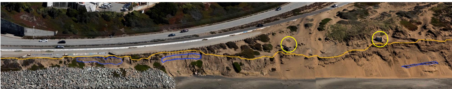
CCR imagery from October 4, 2019 shows further erosion. Much of the historic bank swallow habitat visible in the top image has eroded away. The approximate 2019 bluff line is shown in orange.
