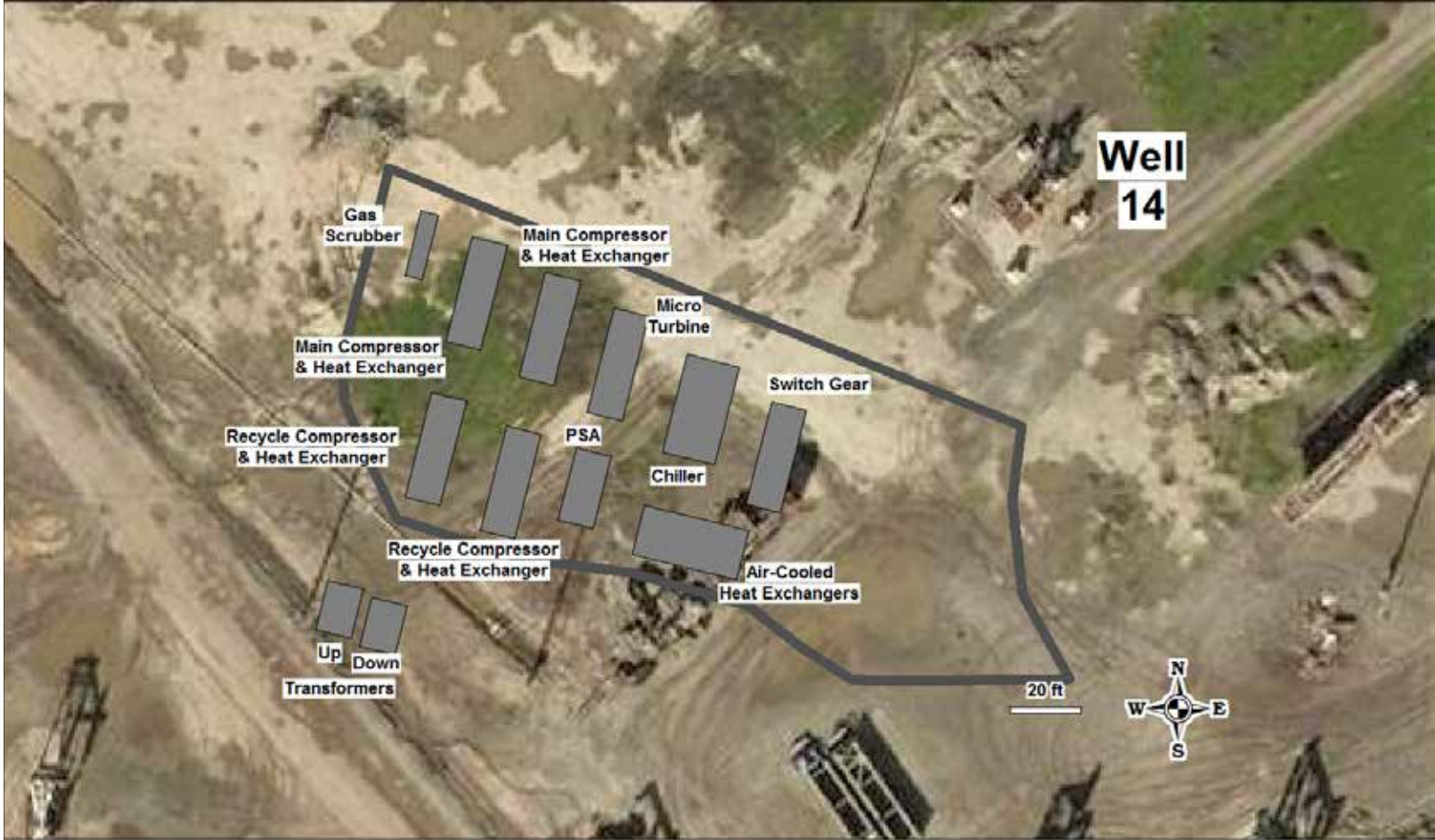
Figure 4 Equipment Layout for the Proposed Gas Plant
