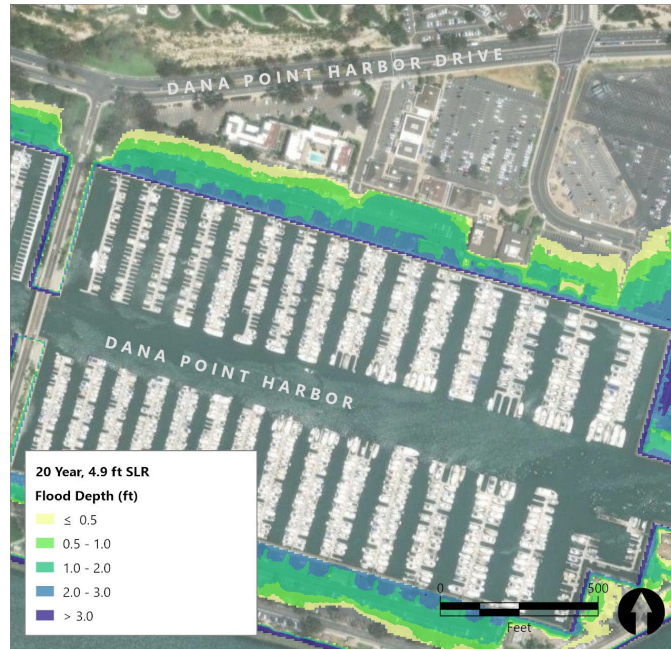
Figure 6 Flood Depths for 20-Year Waves, 4.9 Feet SLR (conservatively above the anticipated +4.5 Feet SLR by 2100)
