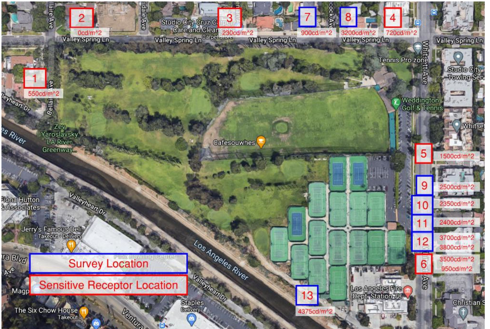
Figure 4 - Existing Conditions Map and Light Measurement Locations
